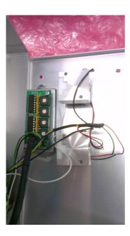
Once removed carefully undo the two screws through the detector plate. Before complete removal note the correct assembly of the components held by the screws. Remove the screws and carefully set aside the wire gauze and spacer, move the fan from the detector block to expose the brass tube mounted in the side of the detector.
