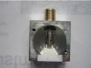
Unscrew the two screws through the white plastic block and carefully ease the detector out and
