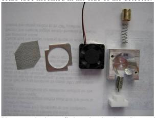
Unscrew the brass fitting slowly, there is a spring inside which holds the detector in place. Remove the brass fitting and spring.
