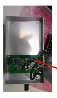
Carefully lift the detector plate from the probe body and disconnect the 5 way connector mounted on the circuit board. Care must be taken not to remove this by pulling on the wires which may cause damage.
