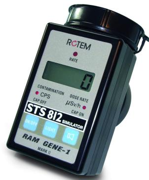
The STS 812 Ram Gene simulator provides a contamination only simulation. To monitor remove the cap, the led will light to show CPS has been selected. The subject may now be monitored by moving the instrument slowly over the clothing keeping the unit within 1 cm of the surface.
