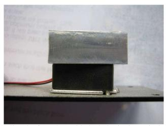
Align the face plate with the holes in the probe body and replace the 10 screws.
