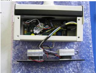
Carefully lift the detector plate from the probe body and disconnect the 5 way connector mounted on the circuit board. Care must be taken not to remove this by pulling on the wires which may cause damage.
